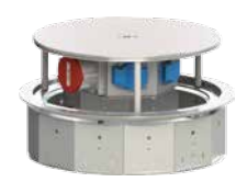
PIANO 9913-Tnw 380x112mm 1x CEE 5/16A, 2x Schuko, 1x RJ 45 double
