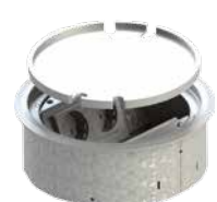
PIANO 9913-Tnw 380x112mm 1x CEE 5/16A, 2x Schuko, 1x RJ 45 double
