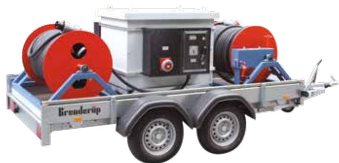
Inspection trolley „3 in 1“ - transformer, big cable reel, trailer, rotary current transformer
