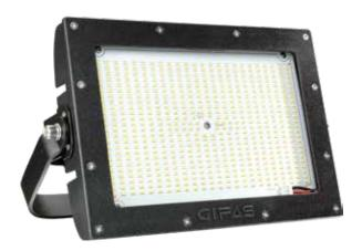
The AlphaLUXX RF -vibration-proof- is developed for special mechanical loads, such as use on moving or vibrating machine parts, conveyor belts or vehicles. Vibration-damped mounting of the ballast and special securing of all screws enable this floodlight beeing robust against vibrations.
