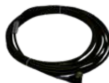
Connecting cable 5m black, angled with socket 3P, IP67, 3 x 0.25mm 2 Item no. 268321
